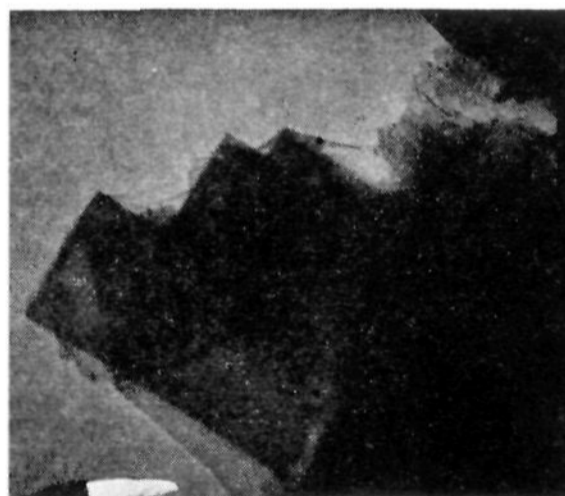
Fig. 6.— \text{SiO}_2:\text{Na}_2\text{O} 11.1:1; magnification 8700; electron microscope.
